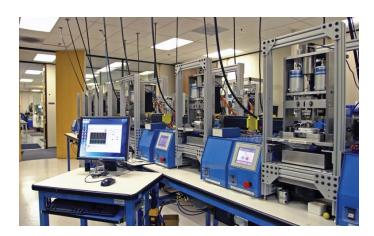
Figure 1: Kinematic wear testing was conducted using custom-built machines designed by Spinal Kinetics
